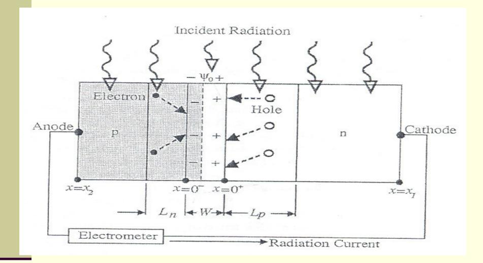
Schematic of a Si pn junction as a radiation detector
