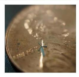
Smitha Rao and J C Chiao designed a tiny windmill that's just 1.8mm thick at its widest point. You can fit 10 windmills on a grain of rice, or hundreds on a typical smartphone case.
