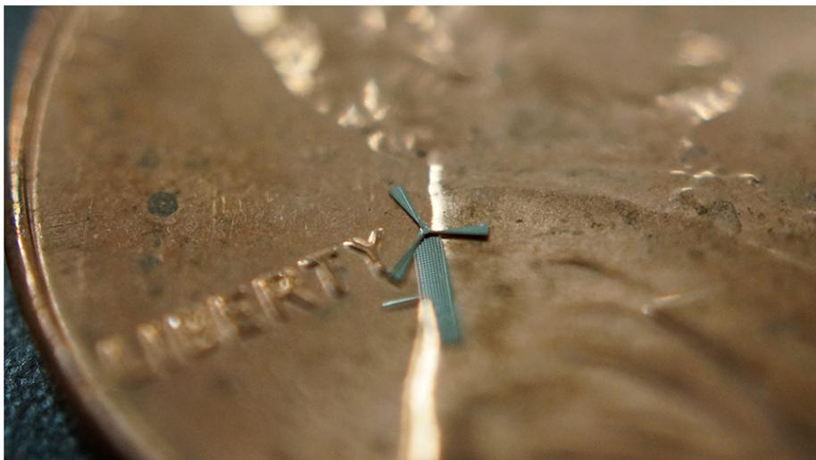
Researchers at the University of Texas at Arlington have come up with a way to build a nickel alloy windmill so small, 10 of them could be mounted on a grain of rice. And if all goes as planned, hundreds of the little things could end up in a case that charges up your smartphone.
