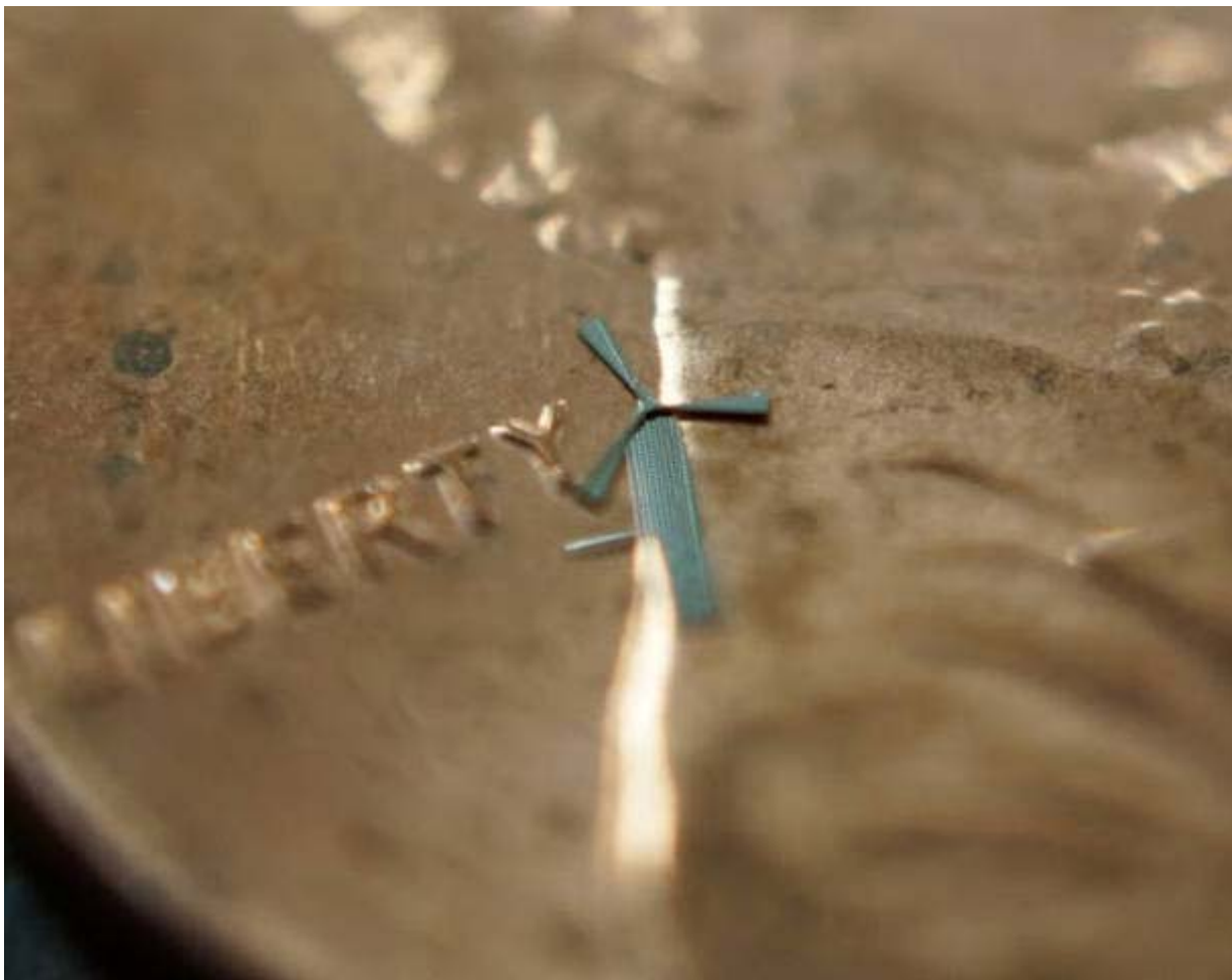
An actual micro-windmill from UT-Arlington, held against a penny.
