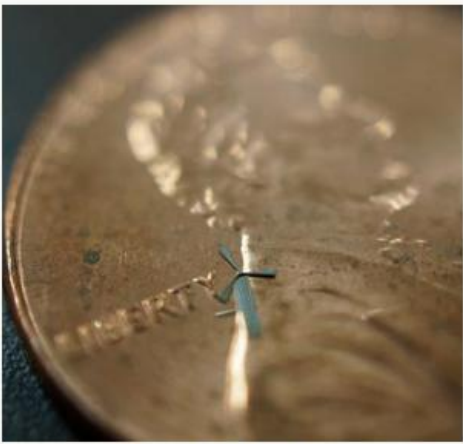
A micro-windmill is pictured on the face of a penny. Photo courtesy of UT Arlington
