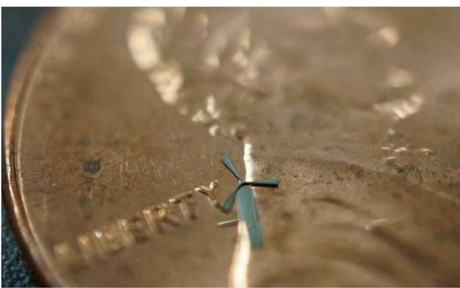
A photo showing a micro-windmill on a penny. Credit: UT Arlington
