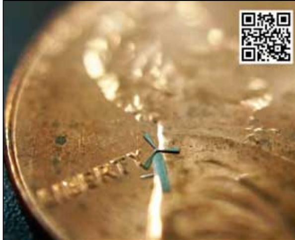
Smitha Rao and J C Chiao designed and built the device that is about 1.8 mm at its widest point. A single grain of rice could hold about 10 of these tiny windmills. Hundreds of the windmills could be embedded in a sleeve for a cellphone.
