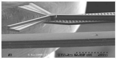
(A detail view of the side of the microwindmill created with an electron microscope. Courtesy WinMEMS Technologies.)
