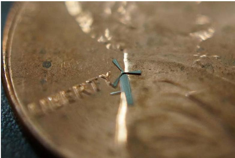
At the University of Texas Arlington, scientists J.C. Chiao and Smitha Rao have developed micro-windmills which recharge smartphones. The miniature device is only 1.8mm wide, which is insanely small. Their thought is that many of the devices could be attached between a small casing, allowing a breeze to come through;
