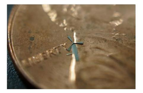
At the University of Texas Arlington, scientists J.C. Chiao and Smitha Rao have developed micro-windmills which recharge smartphones. The miniature device is only 1.8mm wide, which is insanely small. Their thought is that many of the devices could be attached between a small casing, allowing a breeze to come through; hence powering the windmills to create a charge. This is pretty nuts, lets see if anything is to come of it.
