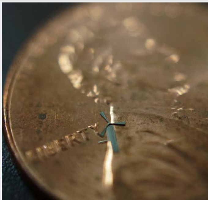
The windmills compared to a penny. The wind generators are bout 1.8mm at their widest point.
