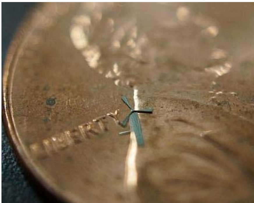
The micro-windmill, shown here on the surface of a penny, developed by University of Texas Arlington researchers. (Credit UT Arlington)
