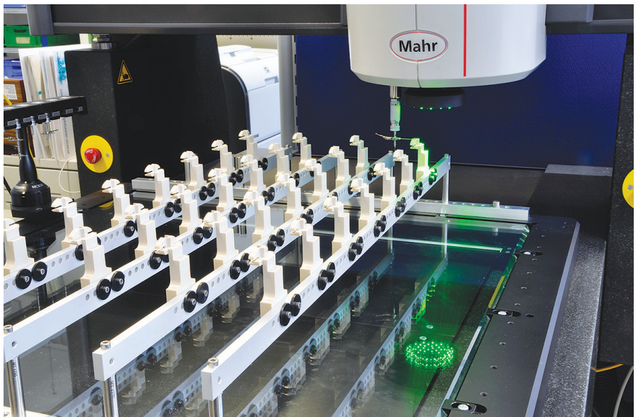
This multisensor system incorporates pallets that allow it to inspect 30 to 40 medical implants in one setup.
