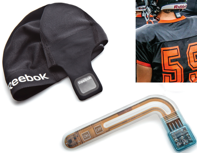
The Reebok CHECKLIGHT sports impact indicator positions wearable electronics directly on the athlete. LED lights illuminate yellow or red depending on severity of impact.
