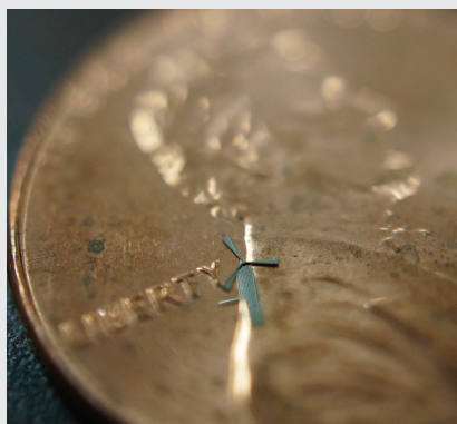
A micro windmill developed at the University of Texas at Arlington.
