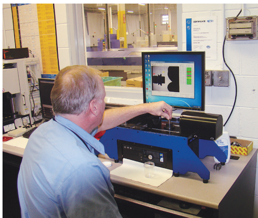
A technician inspects a part using a laser-based measurement system.
