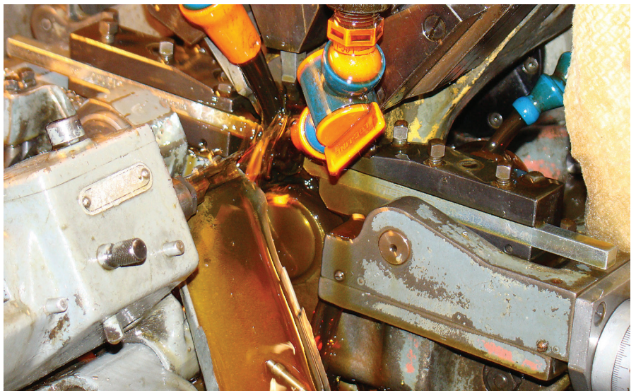
An escomatic in operation at Roberts Swiss.
