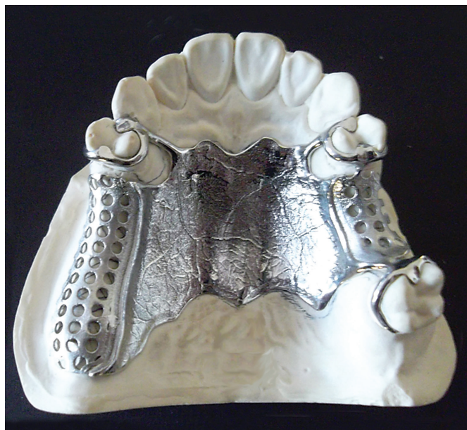
Top view of a dental prosthesis printed using 3D Systems’ ProX 100 dental metal 3D printing system.
