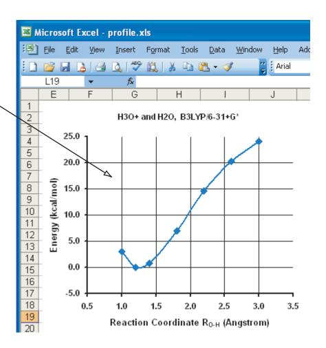
Deprotonation energy of hydronium ion calculated in a presence of a water molecule
