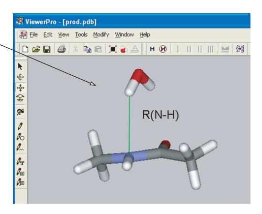
Geometry optimization with a constrained distance
