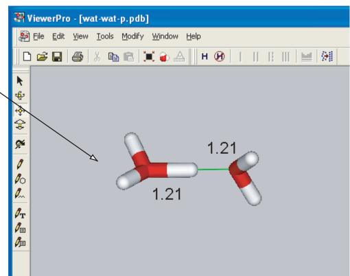
Geometry optimization with a constrained distance and angles
