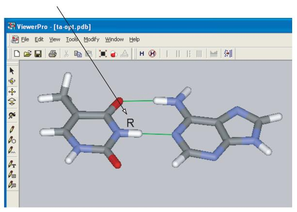
A constrained distance between two atoms
