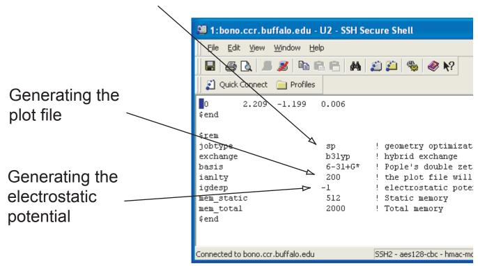
Details of the plot calculations 🕮 1:bono.ccr.buffalo.edu - U2 - SSH Secure Shell Edit View Window Help 📕 🖺 🖺 🦳 🙌 🤌 🛚 🗾 Quick Connect 🛮 📄 Profiles Number of points m<mark>em total</mark> 2000 ! Total memory in the x direction \$plots Electrostatic potential on a grid Minimum and maximum \$end values of the grid in the x direction Connected to bono.ccr.buffalo.edu SSH2 - aes128-cbc - hmac-m
