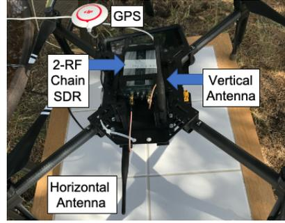
Fig. 1: The spherical coordinate system used in the experiment (a). Both drones are always facing North. The SDR/antenna setup matched for TX/RX (b). Antennas are mounted on the front of each drone.
