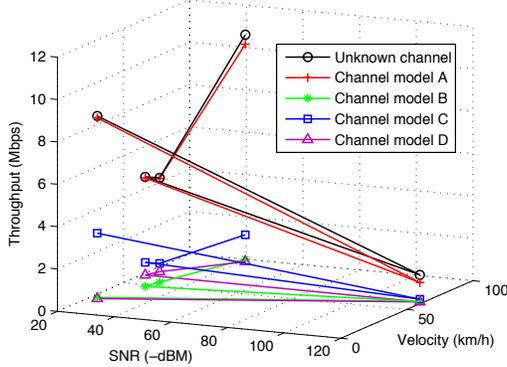
Fig. 2. Throughput versus SNR and velocity for different channel types in 3-D space.
