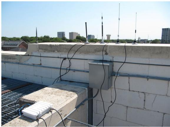
**Fig. 9** Gateworks board with four Ubiquiti radios and antennas at 900 MHz, 2.4 GHz, and 5.8 GHz on top of a parking garage on campus. This figure shows the in-field experiment set-up
