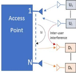
Fig. 1. System model for an IBFD AP that serves multiple users. SI represents the self-interference, U and D represent the uplink and downlink users, respectively.
