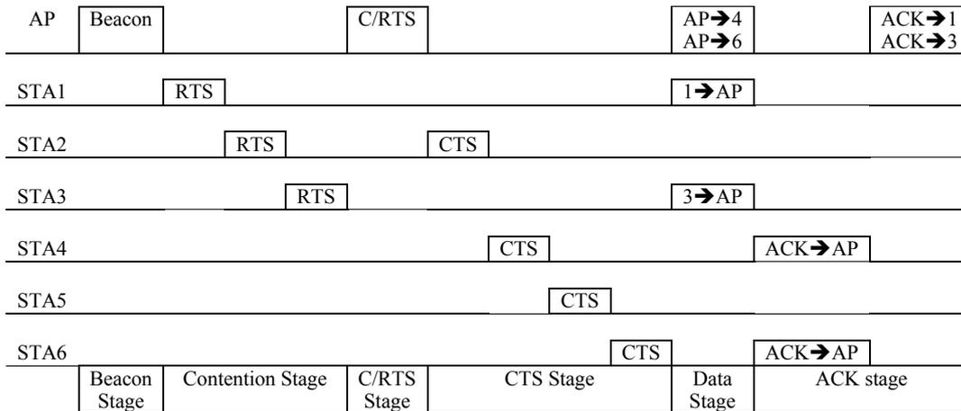
Fig. 3. TFMAC's frame structure. Here, the AP selects users 1 and 3 as uplink users and considers users 2,4,5 and 6 as downlink users by sending a C/RTS frame to these users. Then, the AP finalizes the downlink users selection by using TF-FD, which results in selecting users 4 and 6 in this example.
