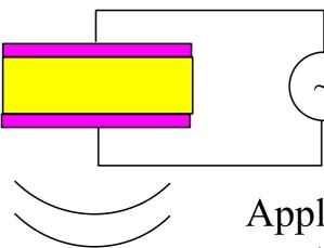
Application of a voltage causes crystal to vibrate at 2-10 MHz.
