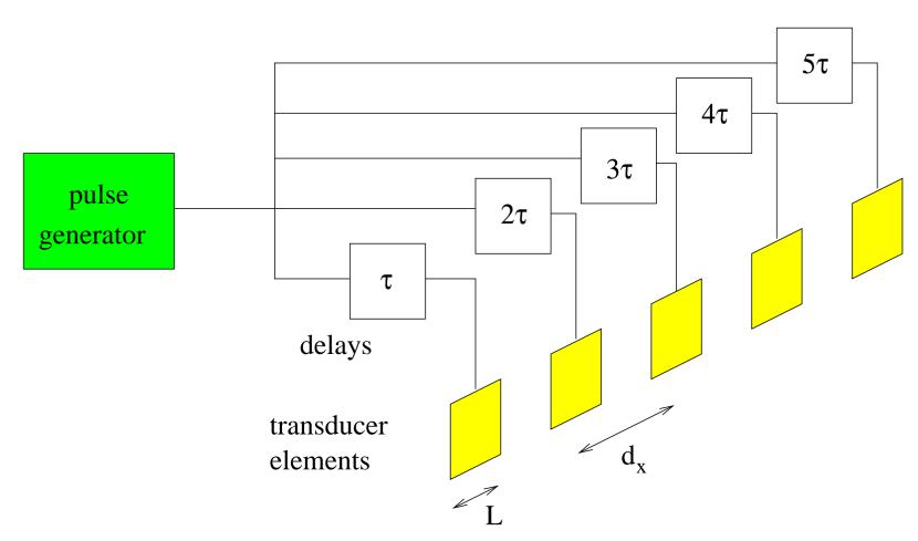
Array can focus and steer the beam over a 2-D region..
