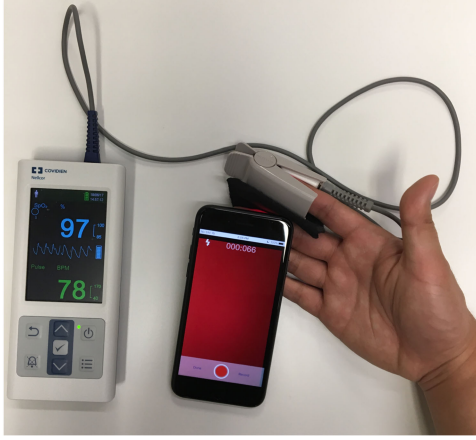
Fig. 1. Experimental setup of ground truth pulse oximetry data collection and custom phone application.
