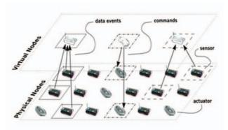
Fig. 1 Virtual sensor concept.
