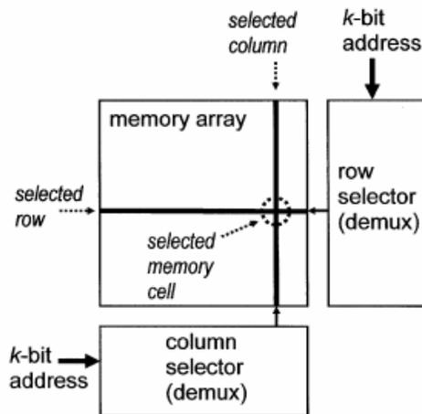
**Figure 3. Nanoscale memory array using crossbar structure [18].**
