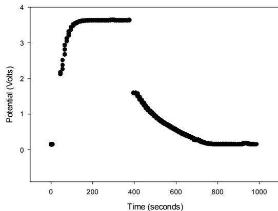
**Figure 2. Charge/discharge data for an individual nanocell.**
