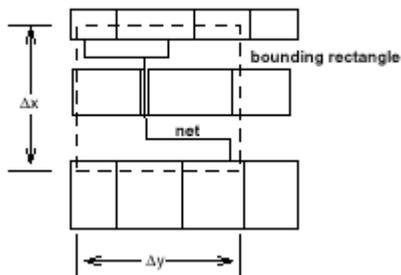
**Figure 1. Half-perimeter wire length of a net.**
