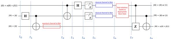
ullet Alice's circuit from time  $t_0$  to  $t_4$  is represented by transfer matrix  ${f T}_0$ :  $\mathbf{T}_0 = (\mathbf{H} \otimes \mathbf{I}_2 \otimes \mathbf{I}_2)(\mathbf{C}_{\mathbf{X}} \otimes \mathbf{I}_2)(\mathbf{I}_2 \otimes \mathbf{C}_{\mathbf{X}})(\mathbf{I}_2 \otimes \mathbf{H} \otimes \mathbf{I}_2)$
