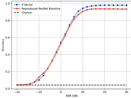
Fig. 1. An overview of the proposed CNN accuracy values for each SNR value in the dataset.
