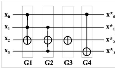
**Figure 1. A cascade of 4 gates with 4 variables**
