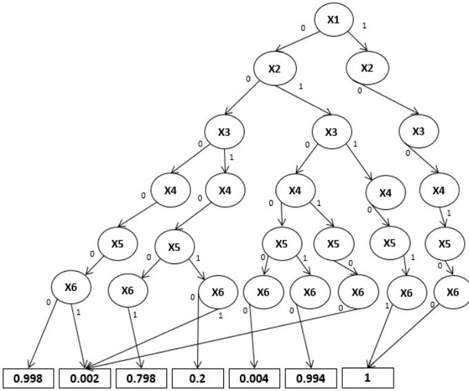
Fig. 5. ADD representation of Fig. 1 communication network
