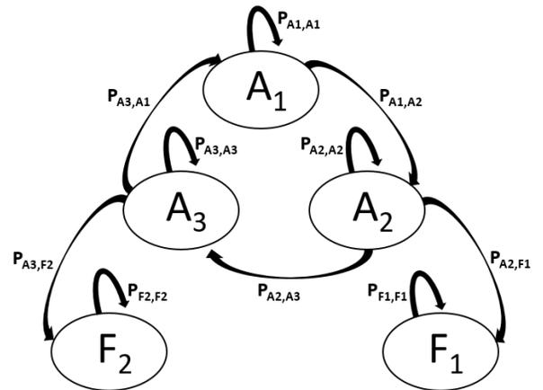
Fig. 2. Markov chain state diagram of example communication network in Fig. 1
