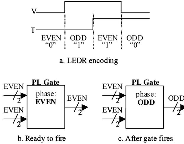
Figure 1. LEDR Encoding and PL Gate Firing
