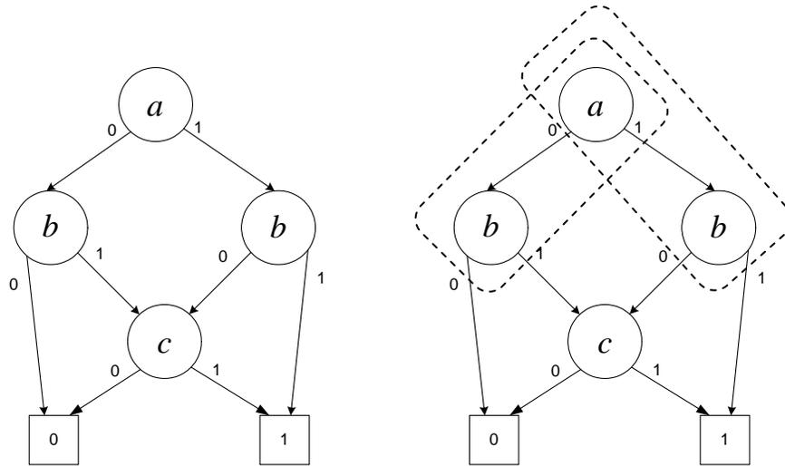
Figure 10. Example BDD for Master Function in Table 1
