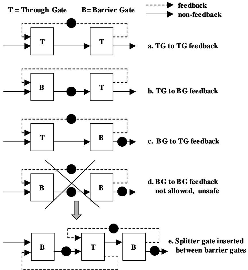
Figure 6: Token marking, feedback insertion, splitter gate insertion rules
