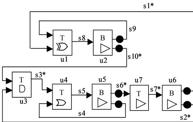
c) PL circuit after splitter gate insertion,  $s_i^*$  indicates an unsafe signal in initial marking
