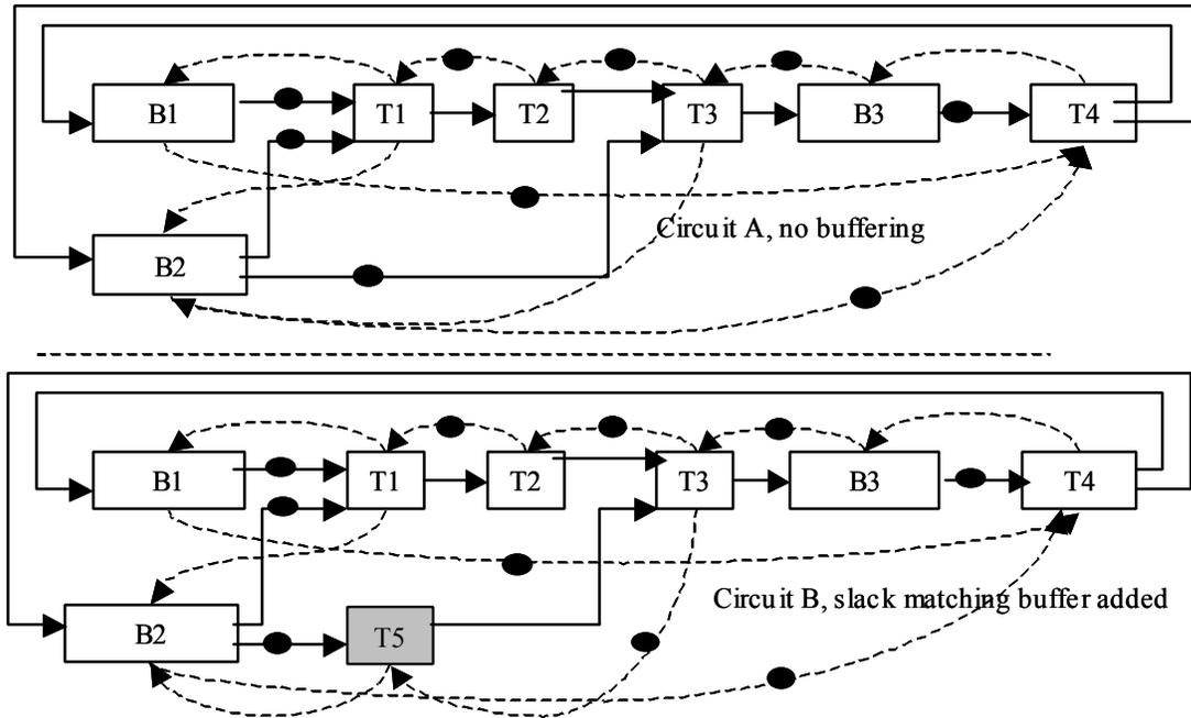
Figure 12. Slack Matching Buffer Insertion
