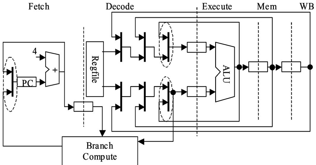
Figure 14. Pipelined CPU
