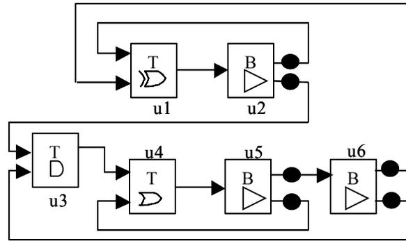
b) PL circuit before splitter gate insertion
