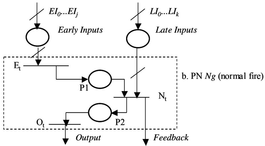
Figure 7. Petri Net models of EGate early and normal fire behaviors
