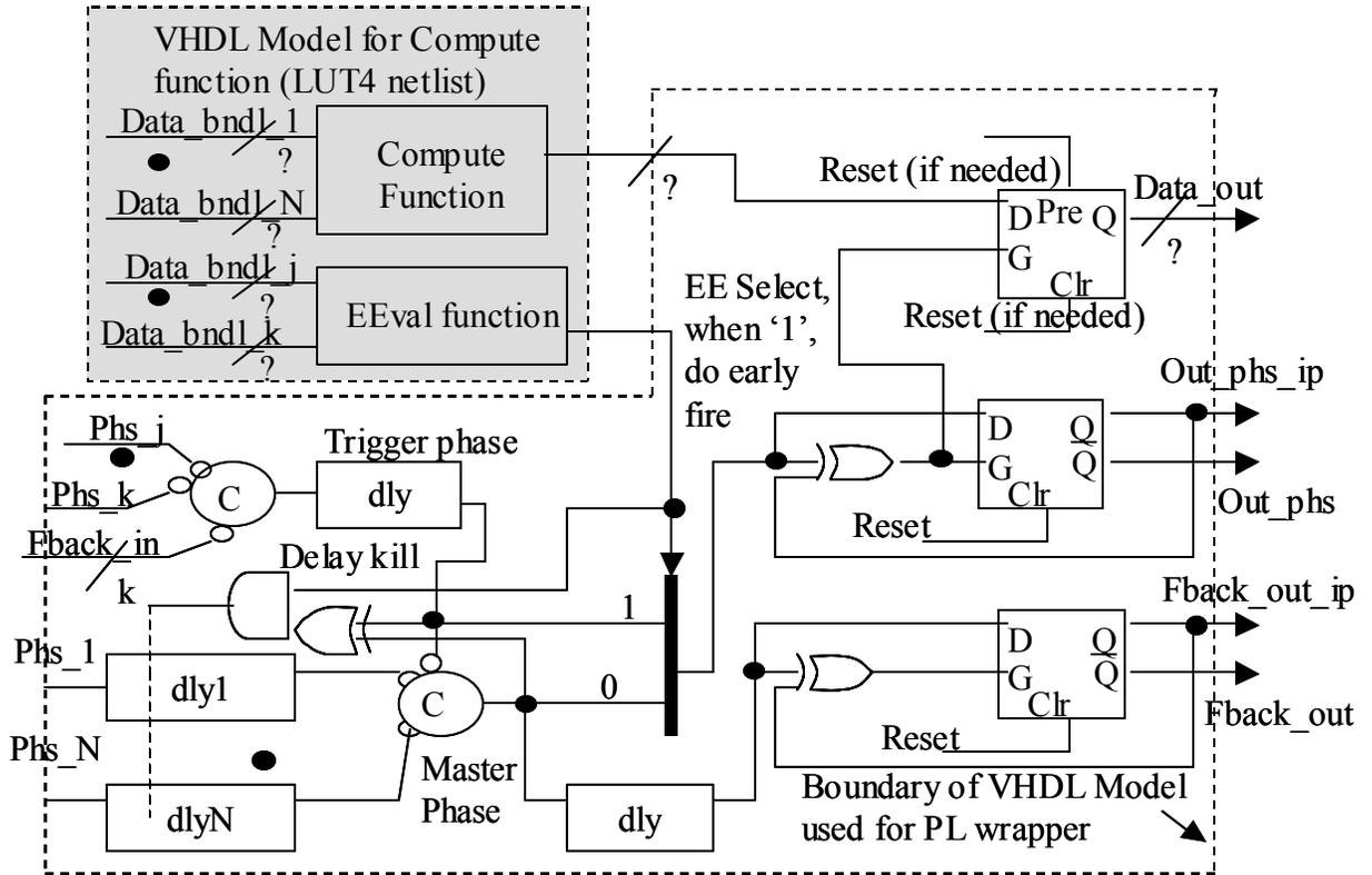
Figure 4. Coarse-grain PL block with early evaluation
