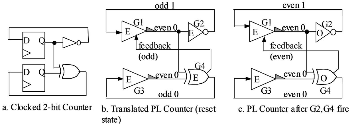
Figure 2. Translation and firing of a 2-bit counter
