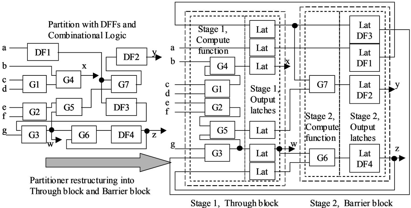
Figure 11. Instance restructuring into Through, Barrier blocks
