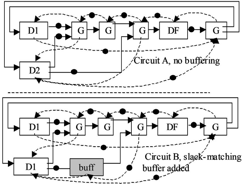
Figure 9. Adding slack matching buffer to improve performance
