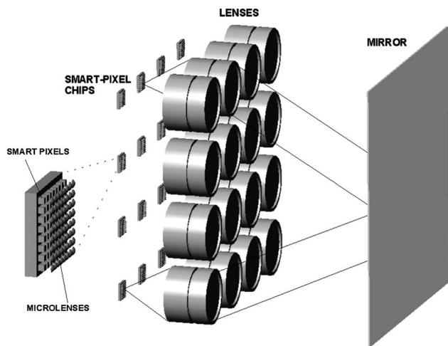
Fig. 1. In the FAST-Net system, a multichip smart pixel array is linked to itself in a global optical interconnection pattern provided by the lens array and the mirror. An optical beam shown depicts the light path between a VCSEL on one of the smart-pixel chips and the corresponding photodetector on another chip.
