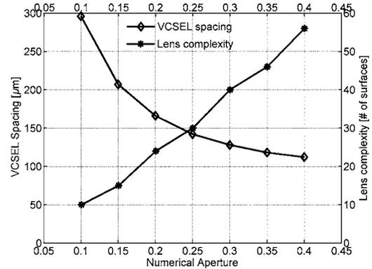
Fig. 6. VCSEL spacing and lens complexity as functions of VCSEL NA for the case *without* microlenses and with a thermal limit of 10 W/cm<sup>2</sup>.
