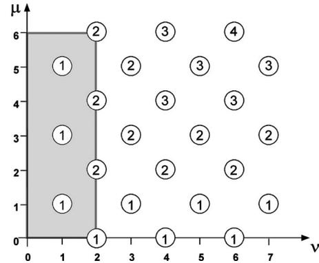
Fig. 4. Rectangle that covers all relevant aberration coefficients for the analyzed FAST-Net system. The aspect ratio of the rectangle depends on the angular imbalance ratio of the system (ratio of the maximum field and aperture angles).
