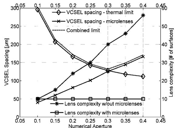
Fig. 8. VCSEL spacing and lens complexity as function of NA for the cases with and without microlenses.
