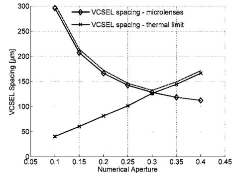
Fig. 7. VCSEL spacing and lens complexity as functions of VCSEL NA for the case *with* microlenses.
