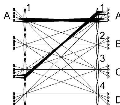
Fig. 2. Schematic cross section of the FAST-Net system showing interconnection pattern between smart-pixel chips. The position of each VCSEL is mapped onto the corresponding beam angle in the space between sending and receiving lenses. After passing through the receiving lens the angle of the beam is mapped back into the position of the focused spot on the receiving chip.
