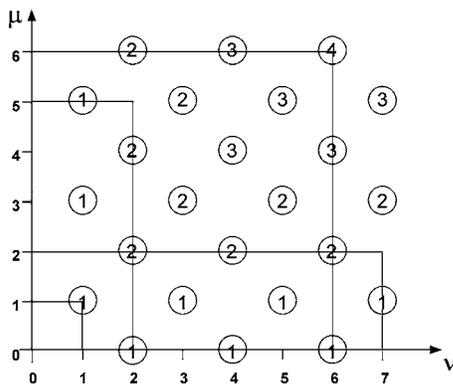
Fig. 3. Graphical representation of the terms of the wave aberration function. Large and small squares and rectangles encompass the coefficients, which are relevant for the typical imaging cases listed in Table 1.
