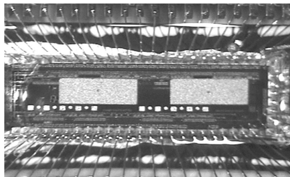
Fig. 15. Micrograph of the chip-on-board packaging, showing that two photodetector arrays are attached to the transceiver chip by the flip-chip process and the hybridized CMOS chip is wire-bonded to the carrier board.
